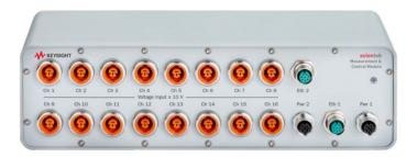
The Scienlab Measurement & Control Module SL1060A from Keysight - Voltage Input ±10 V is a mobile measurement module for measuring voltages (e.g. single cell voltages in battery modules or packs). It features fully galvanically isolated measurement and supply inputs and records all measured values synchronously and with common time stamps by Precision Time Protocol (PTP). The module can be used either as a stand-alone device or as extension for a Scienlab Battery Test System.
