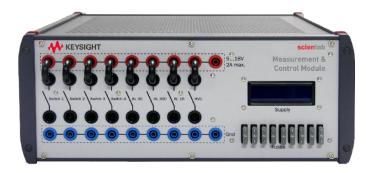
The Scienlab Measurement & Control Module SL1066A – Terminal Control Module provides adjustable voltage outputs for BMS and DUT power supply and floating relay contacts to simulate e.g. vehicle-specific terminals 15, 30 and 31. The mobile module provides fully isolated outputs and allows recording all measured values synchronously and with common time stamps by Precision Time Protocol (PTP).
