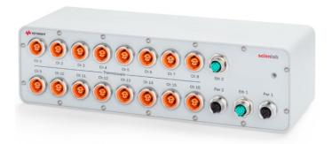
The Scienlab Measurement & Control Module SL1062A – Thermocouple Type K is a portable temperature measuring module for record thermocouple - temperature sensors of type K. It features fully galvanically isolated measurement and supply inputs and records all measured values synchronously and with common time stamps by Precision Time Protocol (PTP). The module can either be used as standalone-device or as an extension of a Scienlab Battery Test System.
