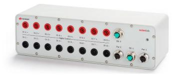
The Scienlab Measurement & Control Module SL1063A – Digital I/O is a mobile measuring and control module for measuring and switching of digital signals. It features fully galvanically isolated measurement inputs and records all measured values synchronously and with common time stamps by Precision Time Protocol (PTP). The module can either be used as stand-alone-device or as an extension of a Scienlab Battery Test System.
